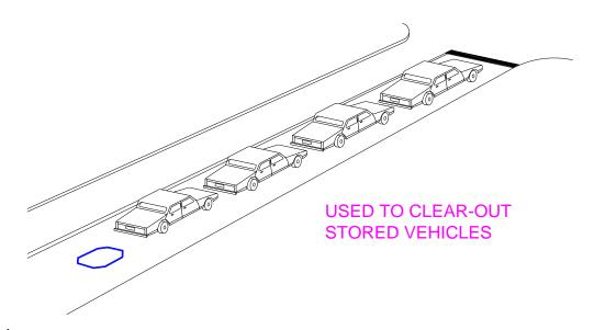
When the detection area is located <u>at</u> the stop line, the purpose of the initial interval is to ensure that a reasonable minimum green time is displayed, not a too-short green time that might violate driver expectation or a too-long green time that is wasteful.
