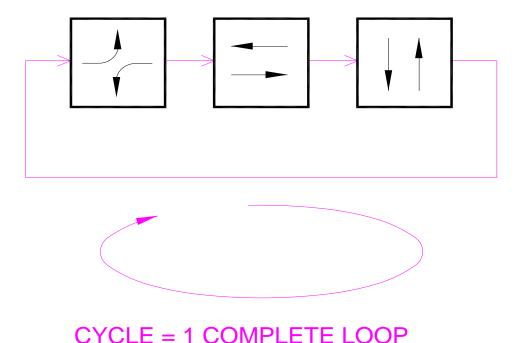
If the three phase combinations in the above diagram each last for 30 seconds, then the cycle length for this signal is 90 seconds. A cycle is sometimes referred to as a "dial" since, in old electro-mechanical controllers, a rotating dial was used to control the timing of the various signal displays. The amount of time during which a particular phase has a green indication (either ball or arrow) is known as the "green interval" for that phase
